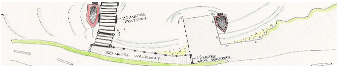
Mainland landing stage and walkway
